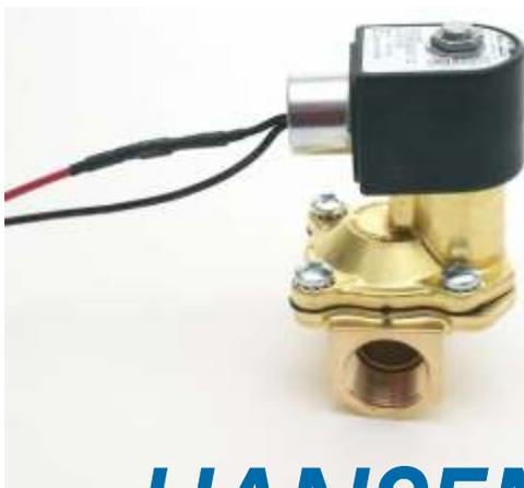
The air stream in the pneumatic duct can be traveling at a very high speed and could carry sparks or embers at this rate. The 901-1 employs a high speed, direct lift solenoid valve which minimizes the total distance required between the detection point on the duct and the spray assembly on the duct.
