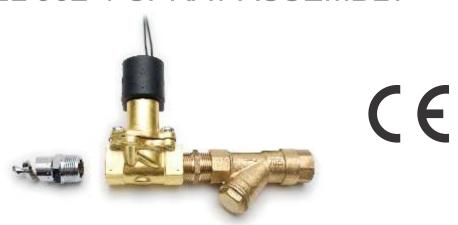
The 902-1 Spray Assembly is designed for deluge of dust collection bag houses. The solenoid valve controlled assembly allows you to mount the valve assembly inside the facility with a dry pipe between the valve and nozzle. This eliminates the need for glycol loops or other expensive arrangements.
